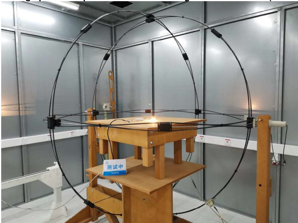
Photograph 2: Set-up for Radiated Electromagnetic Disturbances (Table 3a)
