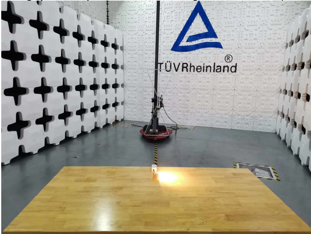
Photograph 4: Set-up for Radio Frequency Electromagnetic Fields Susceptibility (RS)
