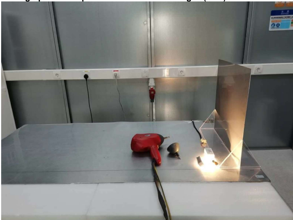
Photograph 8: Set-up for Electrostatic Discharges (ESD)
