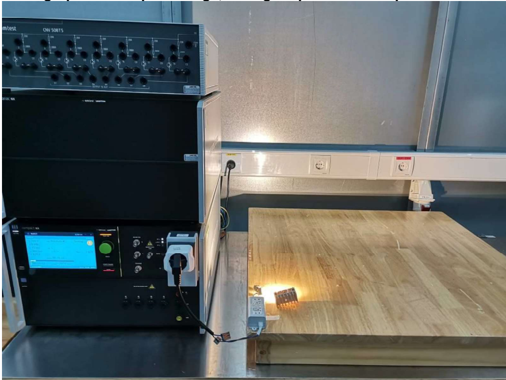
Photograph 8: Set-up for Electrostatic Discharges (ESD)
